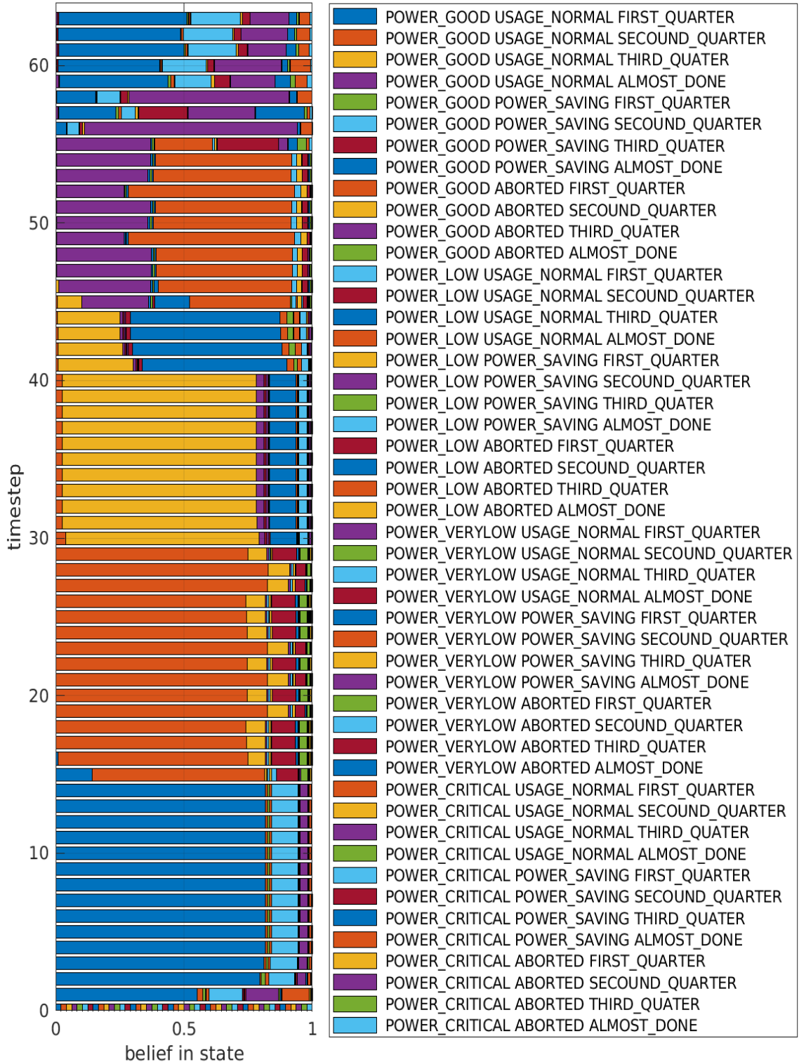
Figure 5-43 Belief distribution for AUV performance with the fault manager: insufficient (Figure 5-42) energy given simulated energy consumption. Belief state progresses with confidence as expected until the last 15% of the mission where the state becomes more uncertain due to the lower energy modes.
