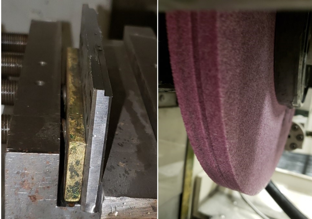
Figure 7.5: Setup for coolant flow groove depth experiments
