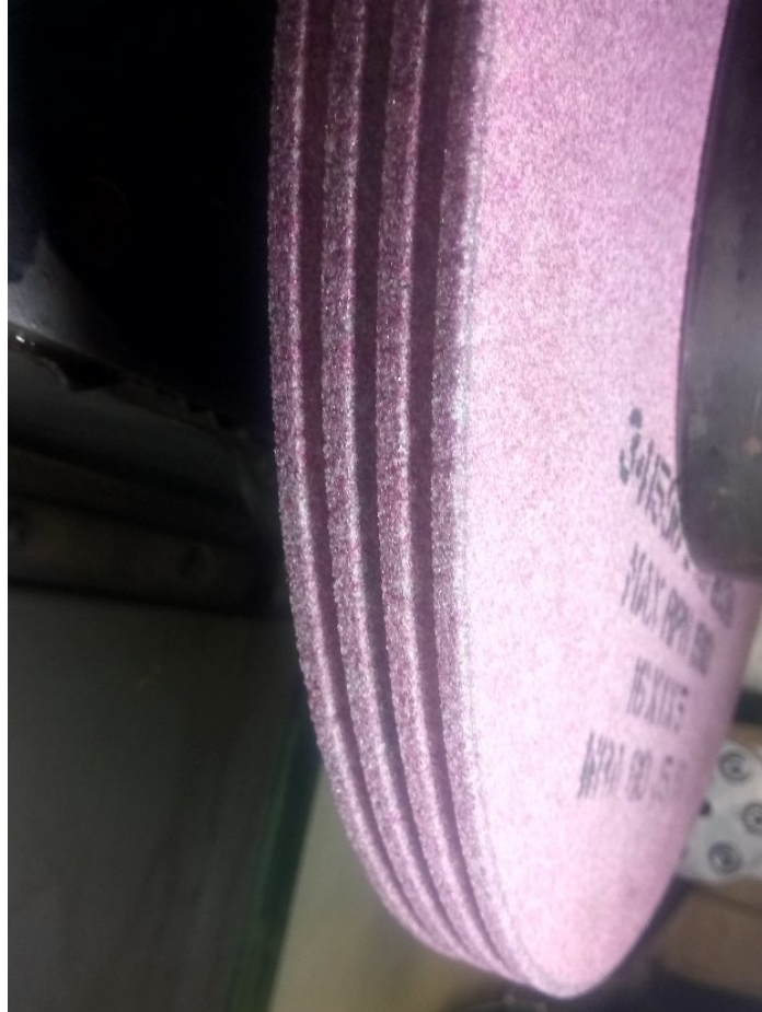
Figure 4.6: Image of grooved grinding wheel
