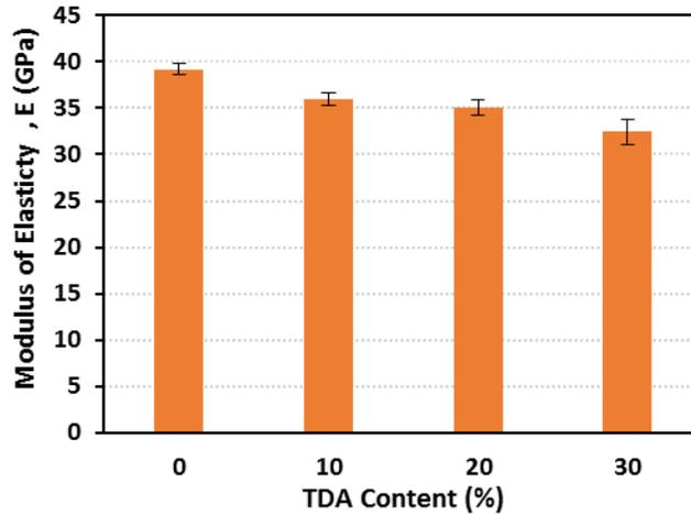
Figure 6. Effect of TDA on concrete elastic modulus
