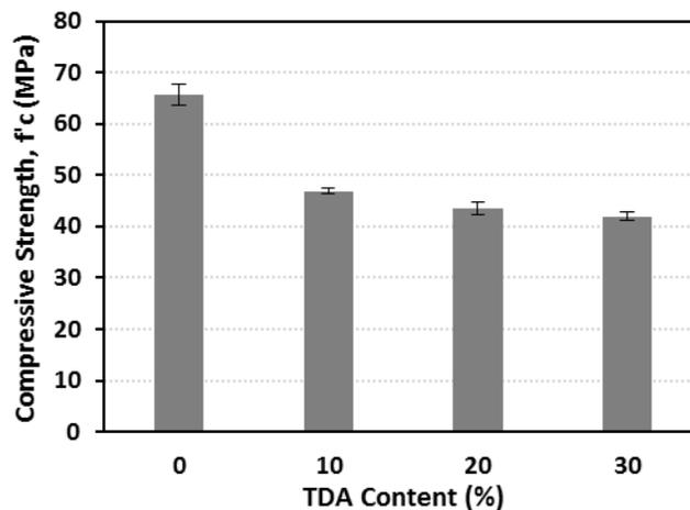
Figure 5. Effect of TDA on concrete compressive strength
