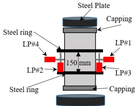
Figure 4: Schematic illustration of the test set-up
