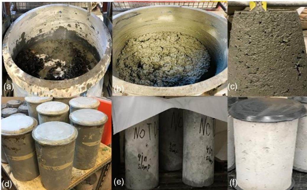
Figure 3: Preparation of concrete specimens: (a) TDA added; (b) mixing the concrete materials; (c) slump test; (d) fresh concrete poured in the cylindrical molds; (e) concrete specimens after curing; (f) capped specimens
