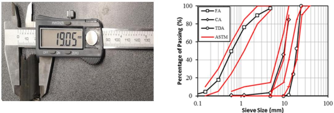
Figure 2: (a) Maximum TDA particle size; (b) Gradation curves for the used materials (Jafarian et al., 2018)
