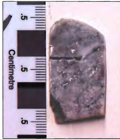
Figure 4.5 This is an example photo of a core chip sample of the MM Quartz Porphyry
