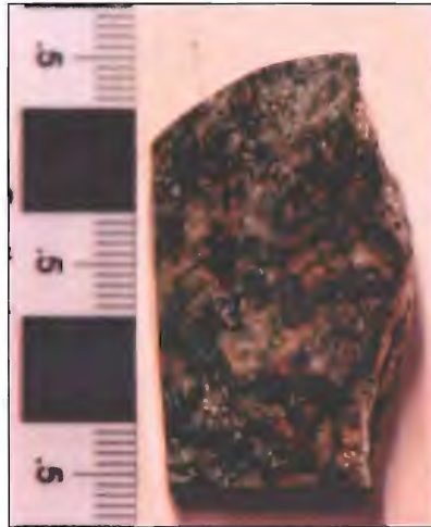
Figure 4.3 This is an example photo of a core chip sample of the MM Granodiorite
