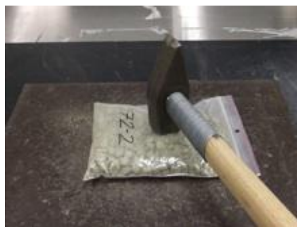
Figure A2: Hammering the sample within its sample bags.
