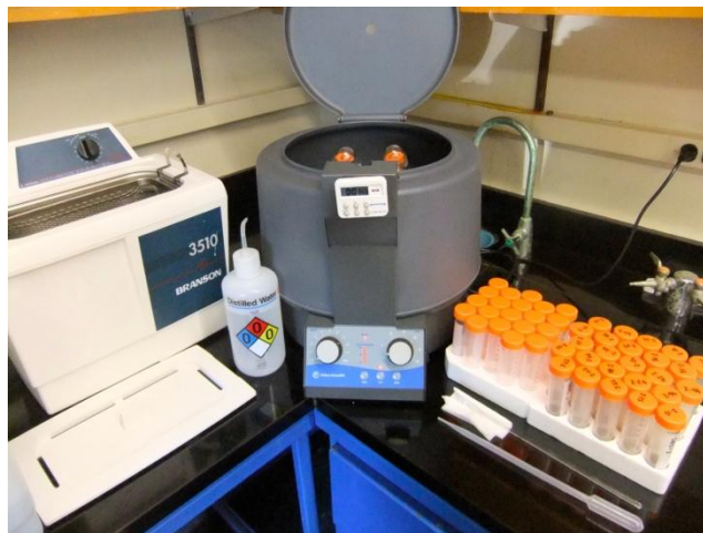
Figure A9: Equipment for rinsing the samples of acetic acid with a centrifuge.
