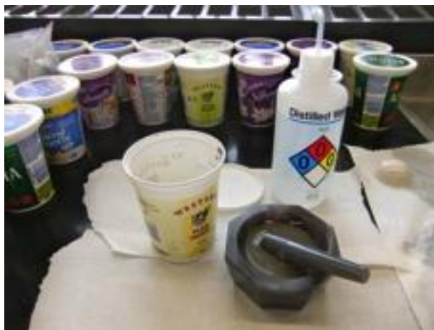
Figure A4: Add soaked sample to mortar and pestle with deionized water.
