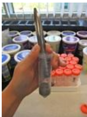
Figure A8: a) 10 mL of sample put into centrifuge vials, b) 80 mL of deionized water with 20 mL of acetic acid to add to it in the fume hood..
