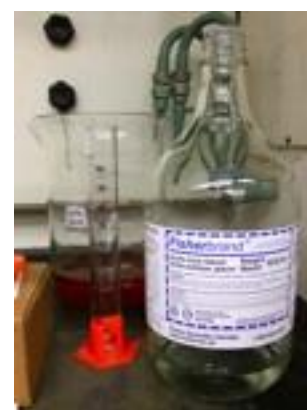
Figure A8: a) 10 mL of sample put into centrifuge vials, b) 80 mL of deionized water with 20 mL of acetic acid to add to it in the fume hood..
