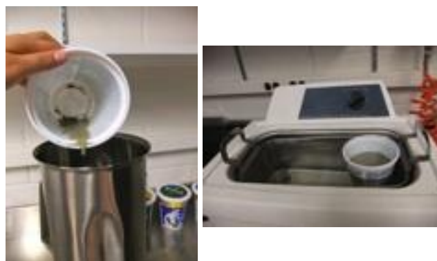
Figure A6: a) pouring the mixed sample into the Waring blender, b) place the sample in an ultrasonic bath for 5 minutes after blended.
