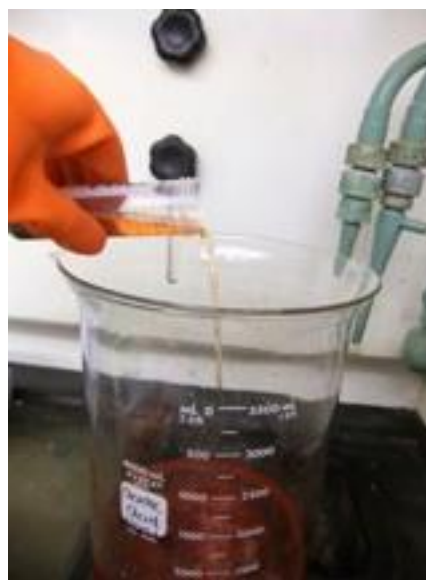
Figure A10: After the first 5 minute centrifuge, decant the supernatant into a labelled acetic acid waste beaker.
