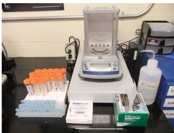
Figure A13: Equipment for weighing in the samples.
