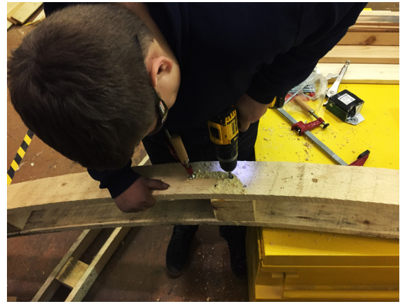
Dawson City youth per-drilling a hole for a carriage bolt.
