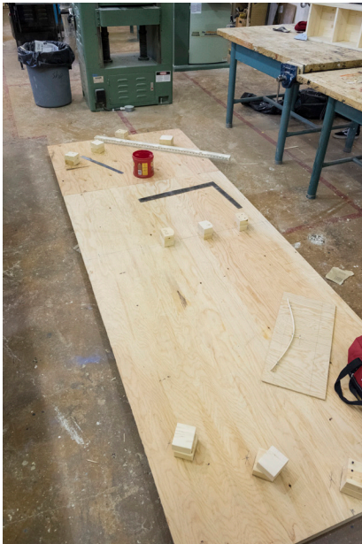
Empty jig with blocks for three sizes of curved beam.
