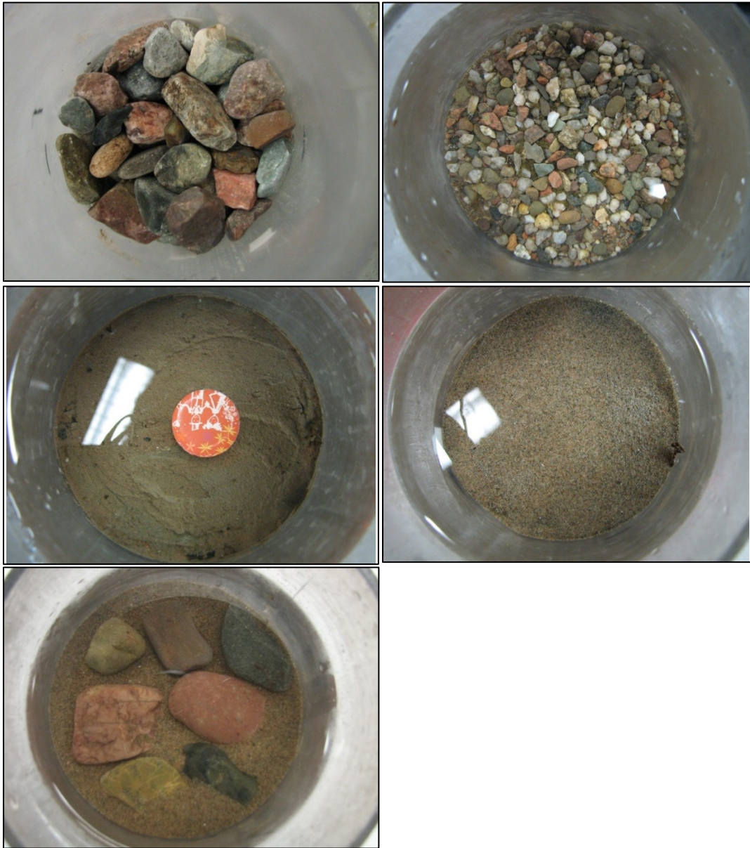
Fig. 1. Downward looking photos onto the bottom substrate used in each of the erosion chamber experiments. In order starting at the top left panel is cobble, sand and gravel, sand, sand and cobble and consolidated mud. The diameter of the cores is the same as that of a slo-core tube, which is 10.8 cm.
