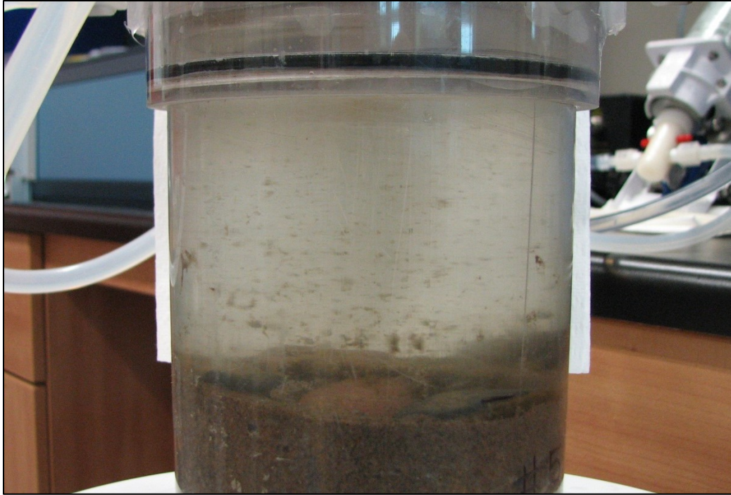
Fig. 3. Photo of a core showing the erosion of waste material at low stress (i.e. 0.08 Pa). The large suspended particles are organic-rich flocs.
