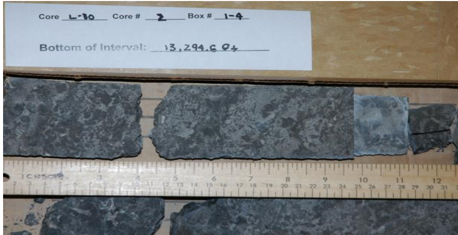
Figure 4.2: Lithofacies B: Wackestone-packstone with intraclasts in a microcrystalline matrix.
