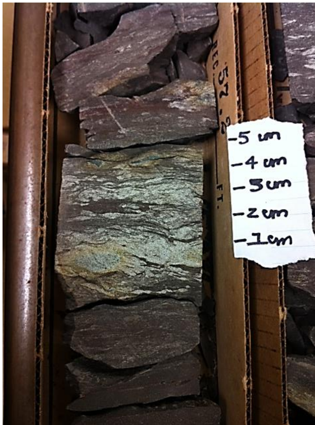
Figure 4.10: Lithofacies 6: Lenticular red shale. White material is lithofacies 1 being mixed with lithofacies 6 and occurring as lenses throughout the lithofacies. Rust color indicates pyrite clasts.
