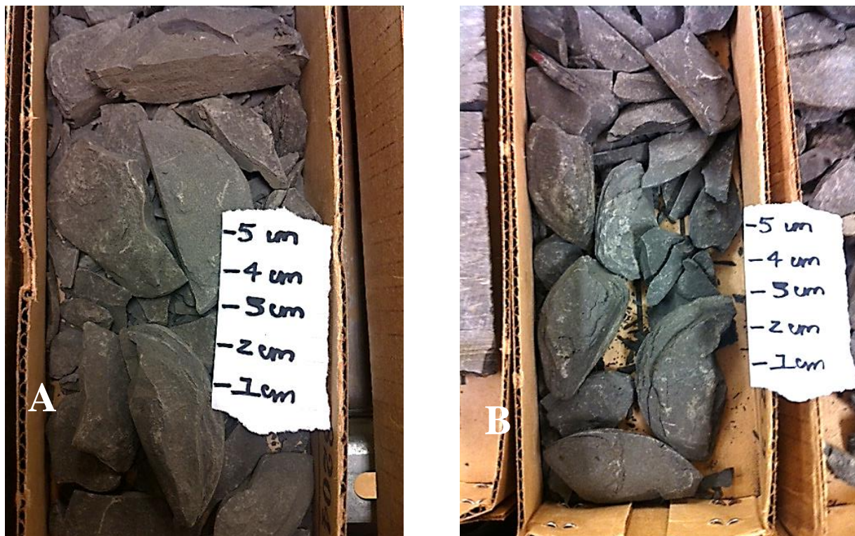
Figure 4. 8: Lithofacies 4: Grey fissile shale. A and B representative of how lithofacies 4 appears at all occurrences.
