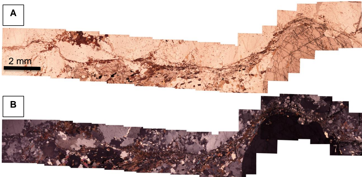
Figure 3.12: Stacked photomicrographs of shear bands consisting of recrystallized quartz and feldspar wrapping a large garnet porphyroblast, in plane polarized light (A) and crossed polarized light (B).
