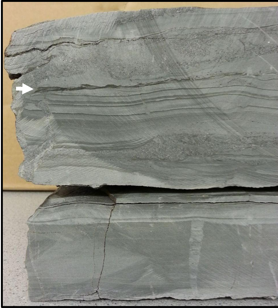
Figure 4.13: Vertical section through the Horton Bluff bedset of sample HBF-1. White arrow denotes dark brown, wavy-crinkly laminae that are less regular than the paler, continuous laminae at other levels, interpreted as mud lenses. Sample is 13 cm tall and 10 cm wide in this photograph. Curved marks are from the saw used to cut the sample.
