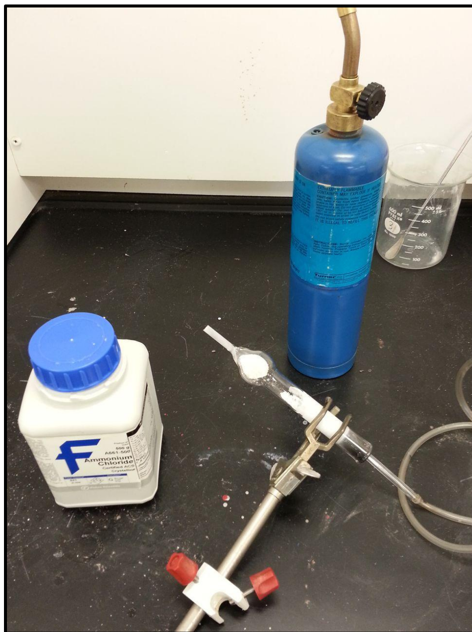
Figure 3.3: Equipment needed for the ammonium chloride process. Under a fume hood at St. Mary's University, Halifax, a butane burner, solid ammonium chloride crystals, glass tube and gripping device for the heated tube. Weak airflow coming through the tube from right to left pushes ammonium chloride gas out of the other end, where the sample would rest several inches away. As the gas exits touching the sample, it sublimates immediately, coating the surface white and making the relief stand out.
