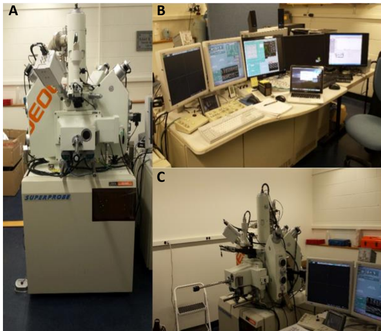
Figure 3.8: (A) Image showing the profile view of the JEOL 8200. (B) Image showing the computer screen array that displayed the camera image and the EMP analyses. (C) Second image showing the different compartments and chambers present on the JEOL 8200.
