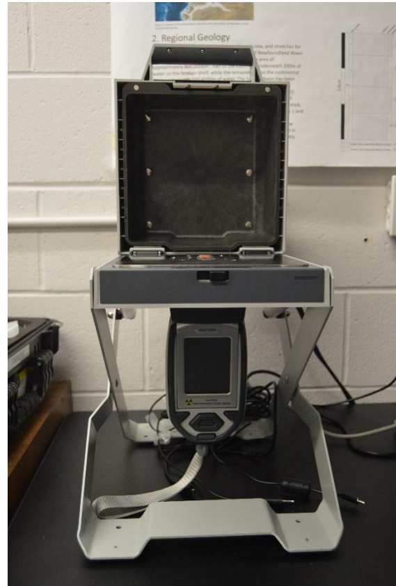
Figure 3.7: XRF gun in desktop configuration with lead lined sample containment chamber open. Samples were placed in the center of the chamber over the XRF detection window.
