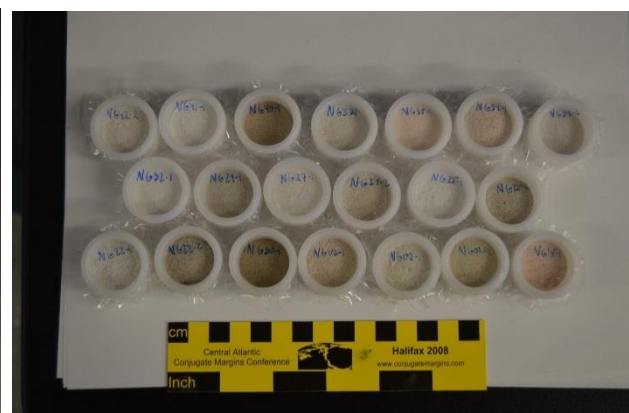
Figure 3.5: Suite of samples in examination vessels after being crushed to a powder, showing different coloured powders based on their variable compositions.
