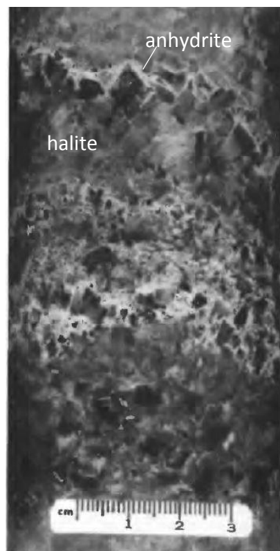
Figure 2.4: Core photograph illustrating snow-on-the-roof texture, where coarse, angular, bottom-growth halite crystals are covered by a thin layer of anhydrite crystals that precipitated out of the water column (Raup & Hite, 1992).
