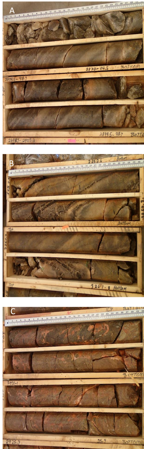
Figure 4.1: Core photographs illustrating; (A) preserved halite banding, alternating between clear and dark halite. The bands dip between 30 and 50 degrees; (B) preserved mudstone beds in a halite dominated succession. Mudstone beds dip between 40 and 60 degrees; (C) brecciated areas within a mudstone dominated succession. Sylvite and carnallite are the dominant precipitate within these brecciated areas as seen by the red-pink coloured mineral that fills the fractures. Four rows, each 0.75 meters long, are shown for each photo.
