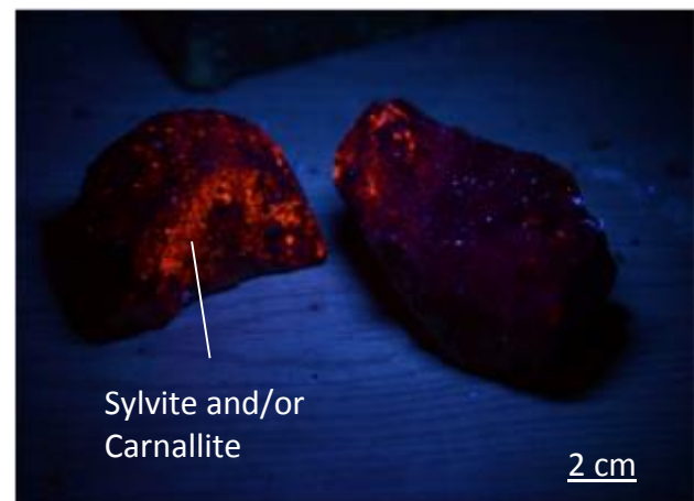
Figure 3.2: Core sample 38 from 913 meters depth, photographed under a UV lamp to illuminate areas of potential sylvite and carnallite concentration, as depicted on photo.
