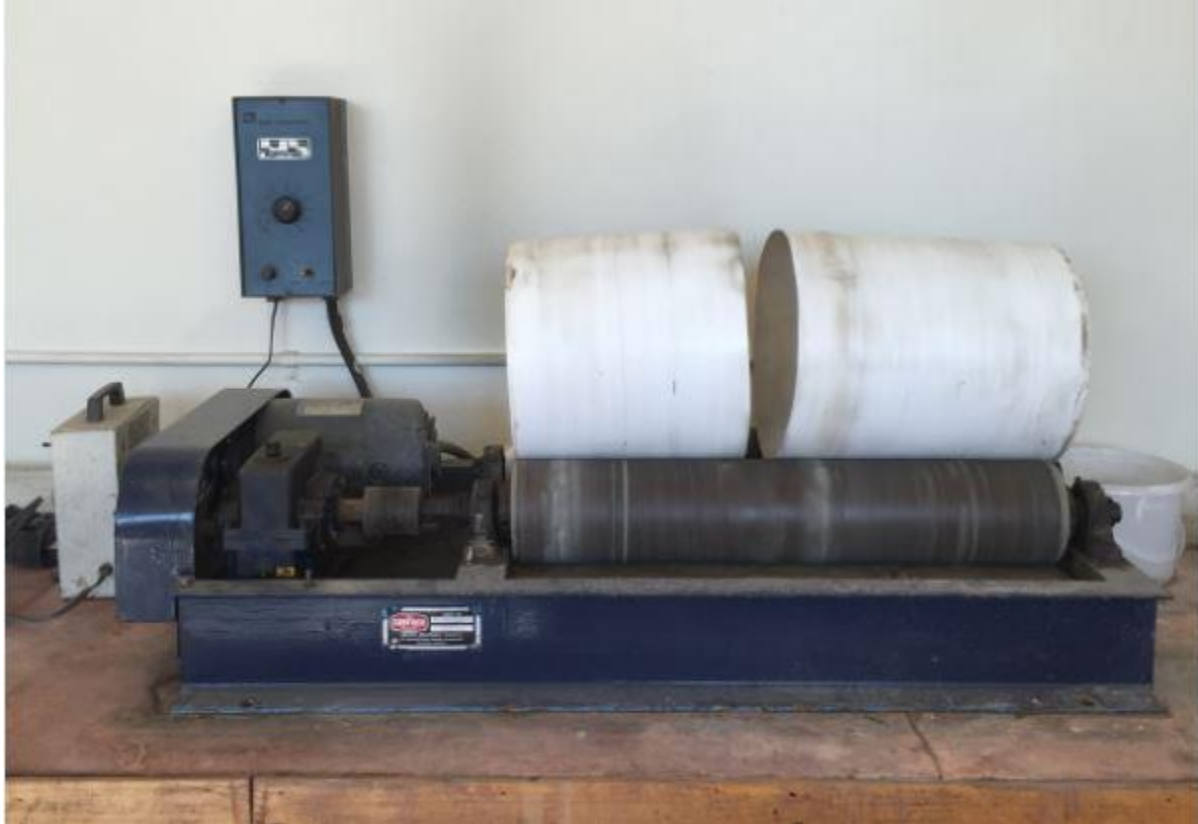
Figure 3.1. The agitation device with two rotating buckets. Each bucket contains four extraction vessels and represents one extraction.
