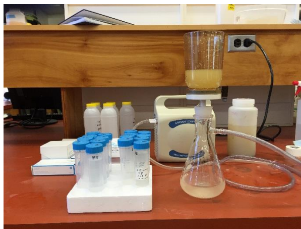
Figure 3.2. Illustrates the filtration procedure. The vacuum is connected to an Erlenmeyer flask and sucking the leachate through a glass filter.
