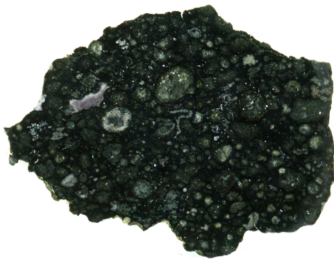
Figure 1: Thin section of Allende CV3 meteorite. Rounded features are chondrules, and irregularly shaped features are CAI's (Calcium-aluminum-rich inclusions)
