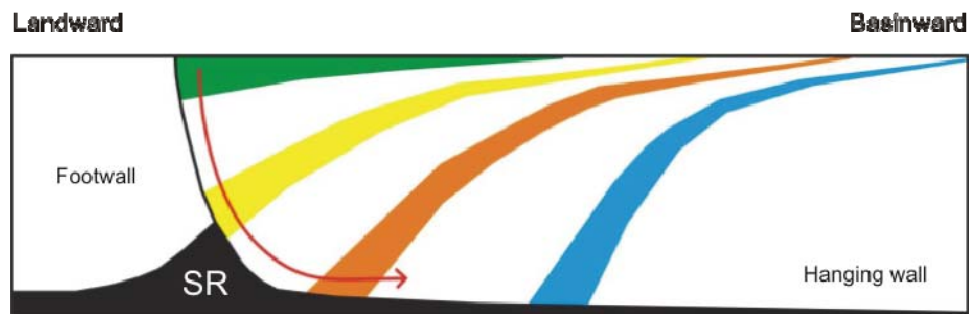
A6. Schematic of a growth fault rollover system with rotation of growing strata (coloured marker horizons) along normal fault indicated by red arrow. SR indicates a salt roller located below the growth fault rollover system. (Modified from MacDonald, 2007).
