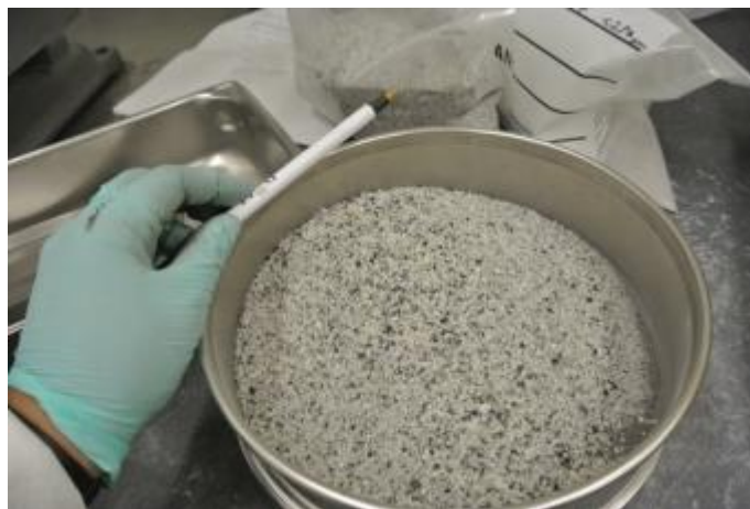
Figure 17: Sample CC07 being sieved after three runs in the disk mill.
