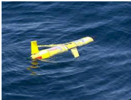
Figure 1.1: A remotely piloted glider off Nova Scotia. Used by OTN to sample the ocean environment.
