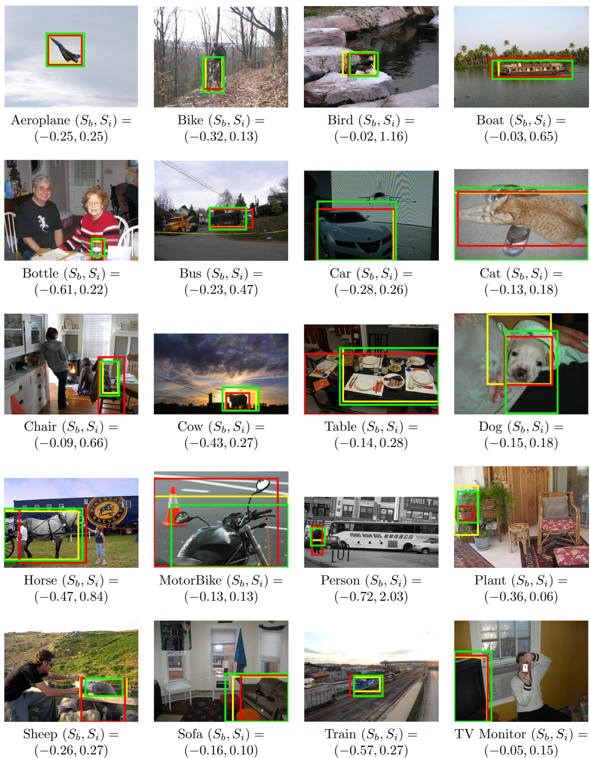
Figure 6.12: Samples of ground truth object (Red) along with output images from RCNN (Yellow) and GT_Loc (Green). Comparing the detection scores of RCNN ( S_b ) and GT_Loc ( S_i ) represents the affect of more precise localization of the proposed method in the object detection.
