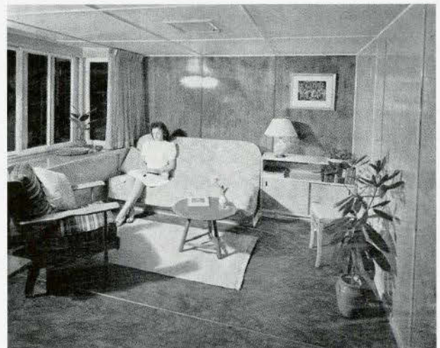
Fig. 10—Living Room of a T.V.A. House with plywood wall finish and linoleum flooring.
