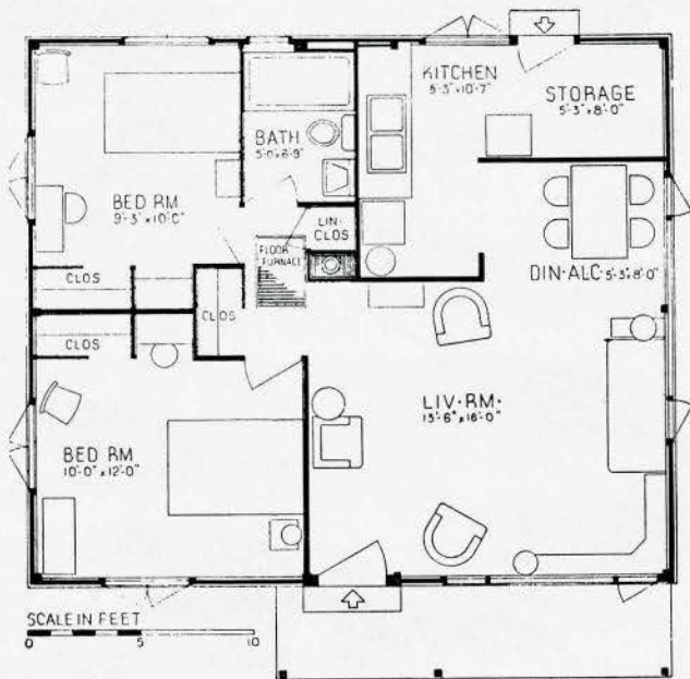
Fig. 6—Plan of "Cemesto" House developed by the John B. Pierce Foundation and built by the Celotex Corp. for the Glen Martin war housing project.
