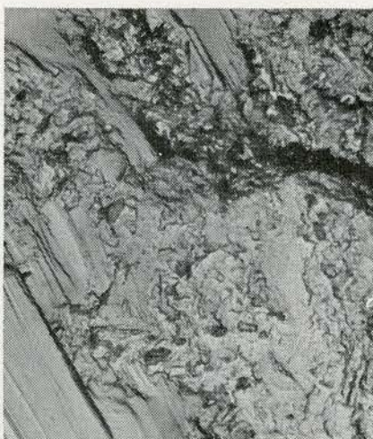
7 Stratified intergrowth of gel and calcium hydroxide. Fracture surface, 4200X
