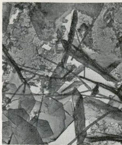
4 Coexisting calcium aluminate trisulfate hydrate calcium aluminate monosulfate hydrate in cement paste. Cut surface, 4200X
