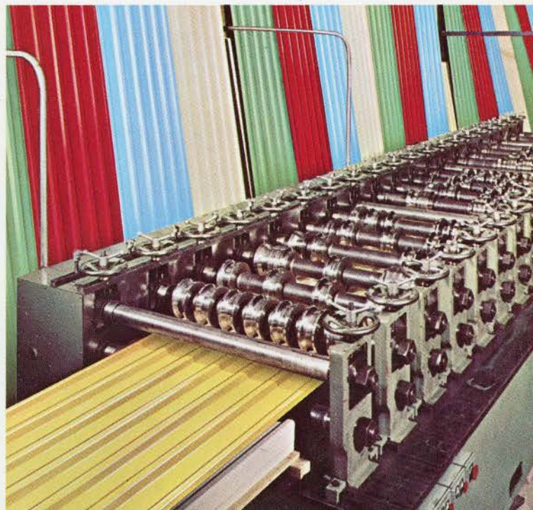
Panels being roll-formed at Eastland Metals Ltd ↓
