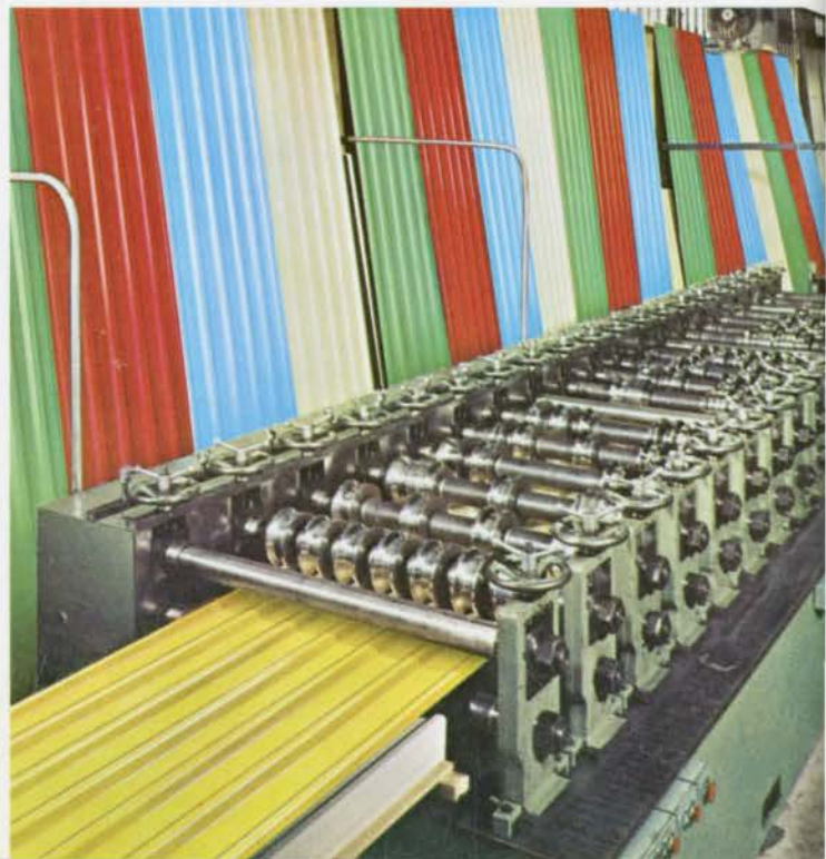
Production inspection at Armco Drainage & Metal Products of Canada Ltd. new roll-forming equipment.
