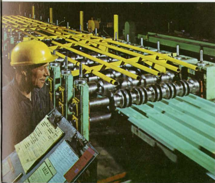
Roll forming at Butler Manufacturing Company (Canada) Ltd.
