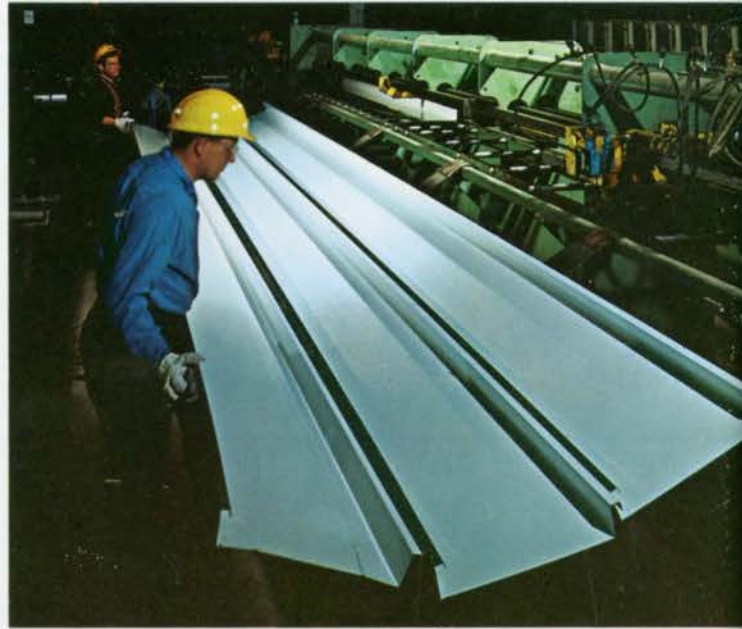
Production inspection at Armco Drainage & Metal Products of Canada Ltd. new roll-forming equipment.
