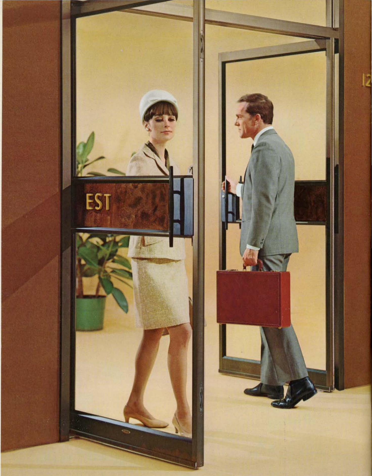
STYLE LEADER 125 ENTRANCE. Unlimited options in center identification panel, using any quarter-inch thickness material . . . wood, porcelain, plastic, glass. Permits customizing of standard doors. Each 125 has weathering on all 4 sides. Top and bottom locking bolt eliminates cut-out in door stile. Closer concealed in transom.
