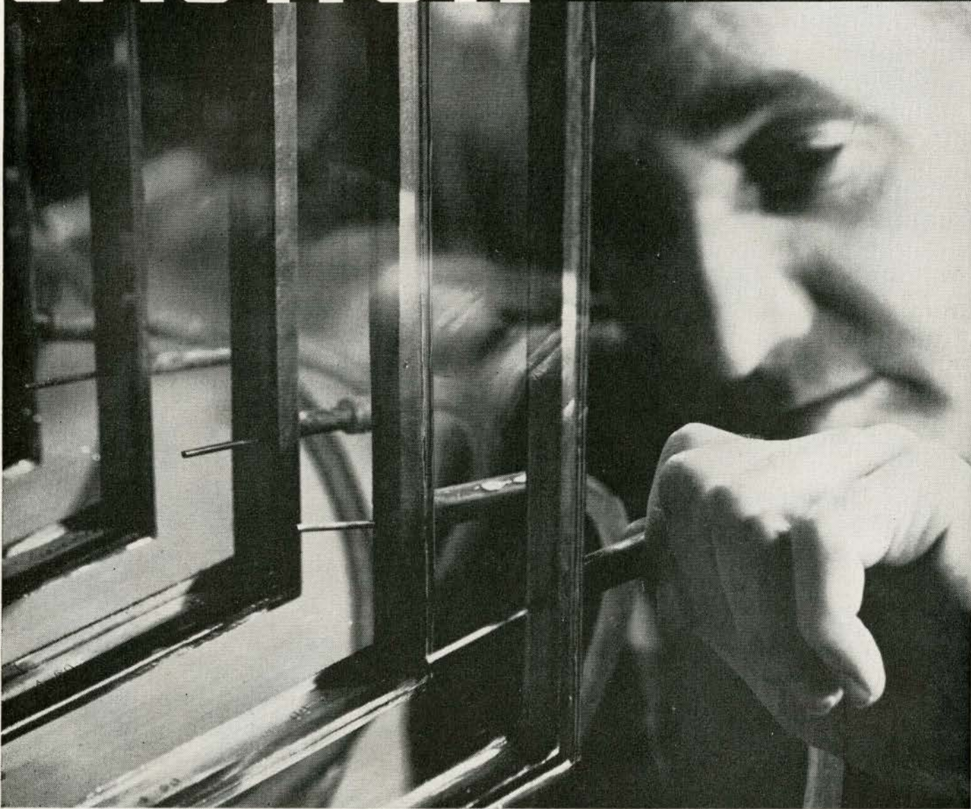
Preparation of Dry Air Space in Thermopane Unit
