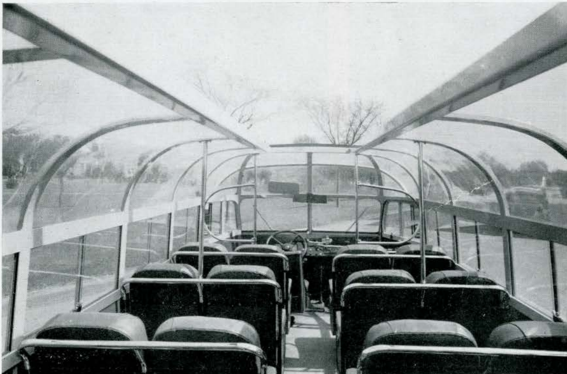
AUTOBUS with acrylic plastic panels for Western Auto and Truck Body Works Ltd., Winnipeg.
