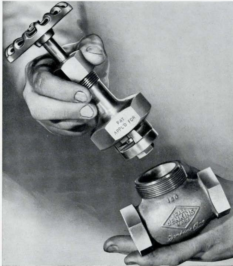
FIG. 106-A, Screwed, Jenkins Standard Bronze Globe Valve, with one-piece screw-over bonnet, and slip-on stay-on disc holder. For 150 lbs. steam working pressure, or 250 lbs. oil, water, gas working pressure.
