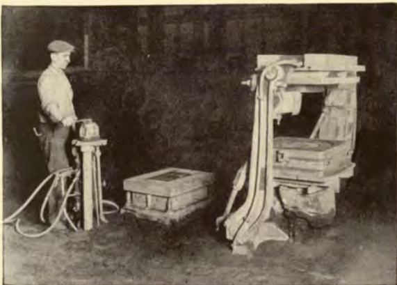
The mould is carefully drawn away from the pattern, assisted by the action of an air-operated vibrator, thus eliminating the irregular tapping operation of the hand moulder.
