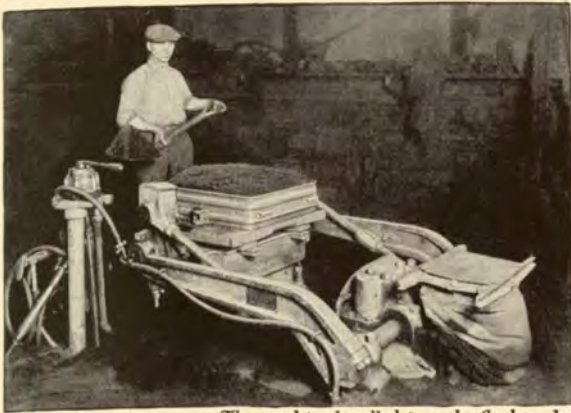
The sand is shovelled into the flask and the mould is then rammed by the air-controlled mechanical jolting of the machine, more evenly than it could be done by hand.
