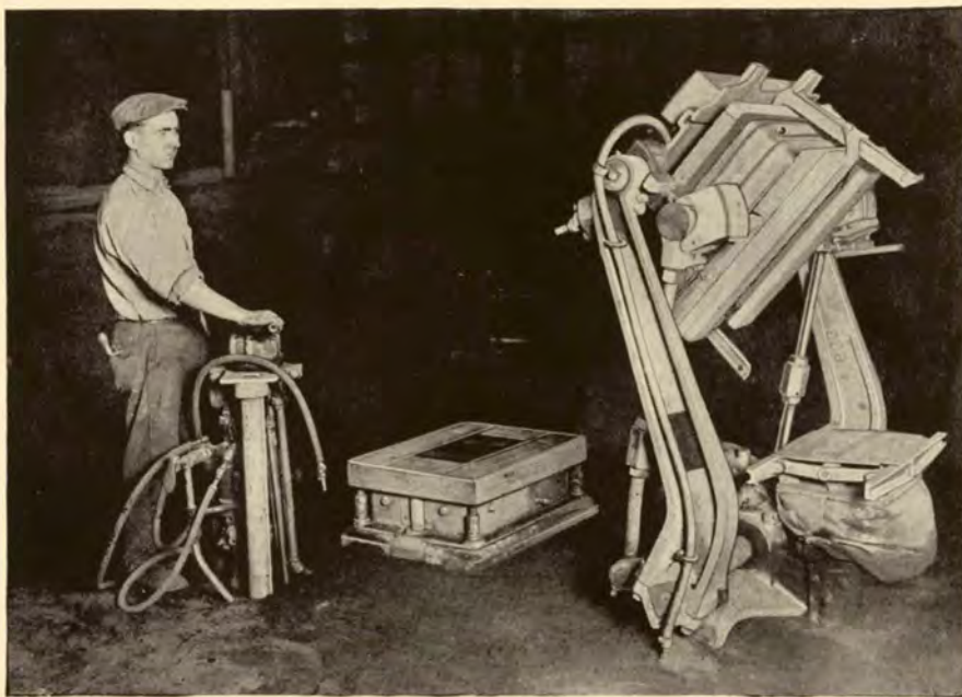
Without the back-breaking effort of hand-moulding methods, the whole flask is rolled over by a light pressure on the control lever.
