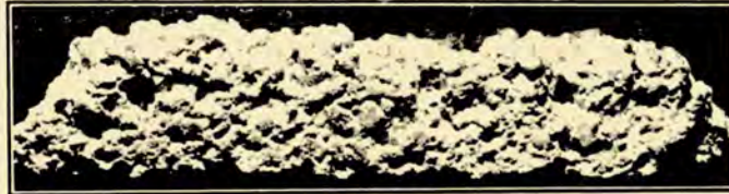
Photograph through magnifying lens showing section through "DEKOOSTO" Acoustic Plaster Note the cellular characteristics right through the whole mass of the plaster to permit the absorption of the sound waves.
