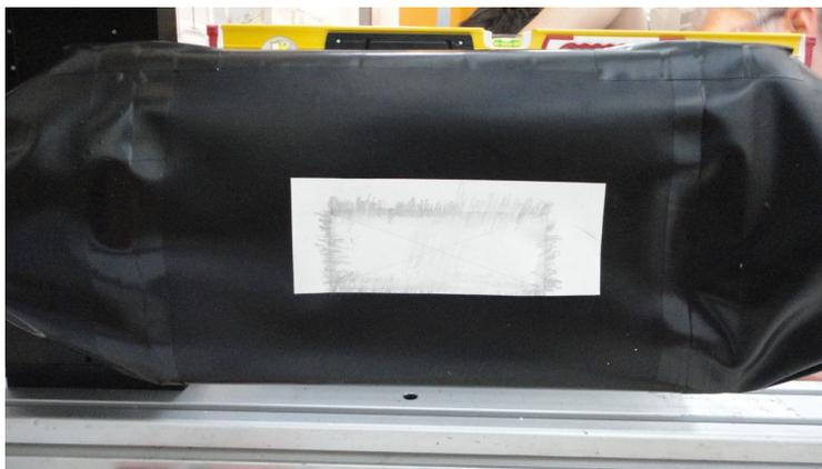
Figure 2.10: A photograph of the veto plastic scintillator.
