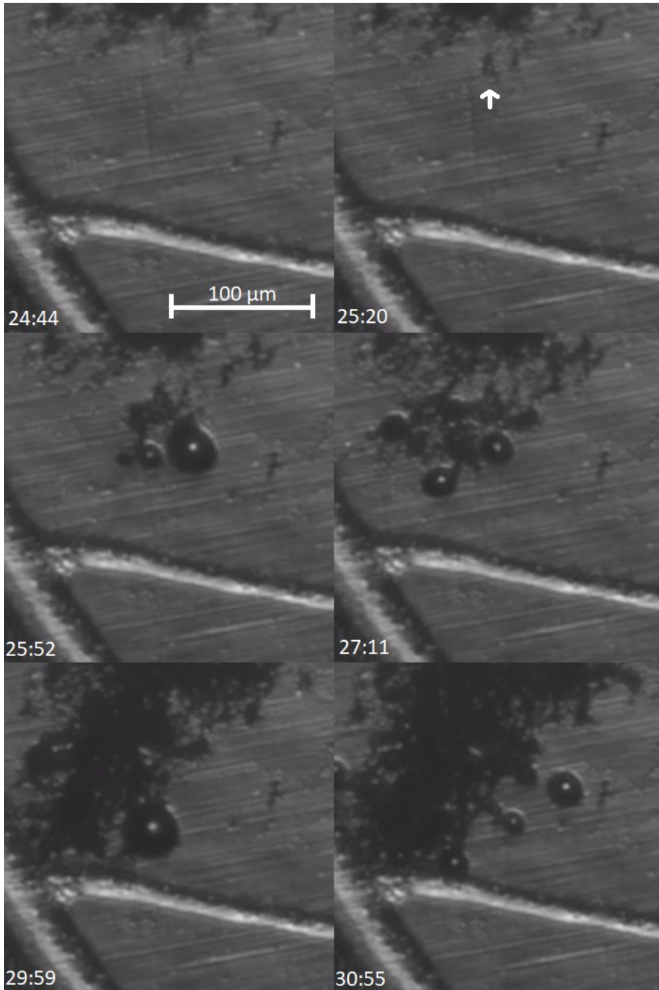
Figure 3.10 Images of the corrosion of a 1 \mu\text{m} Al 5052 sample with flow activated. The arrow indicates the original location of corrosion propagation. The stamps time are given in units of minutes:seconds.
