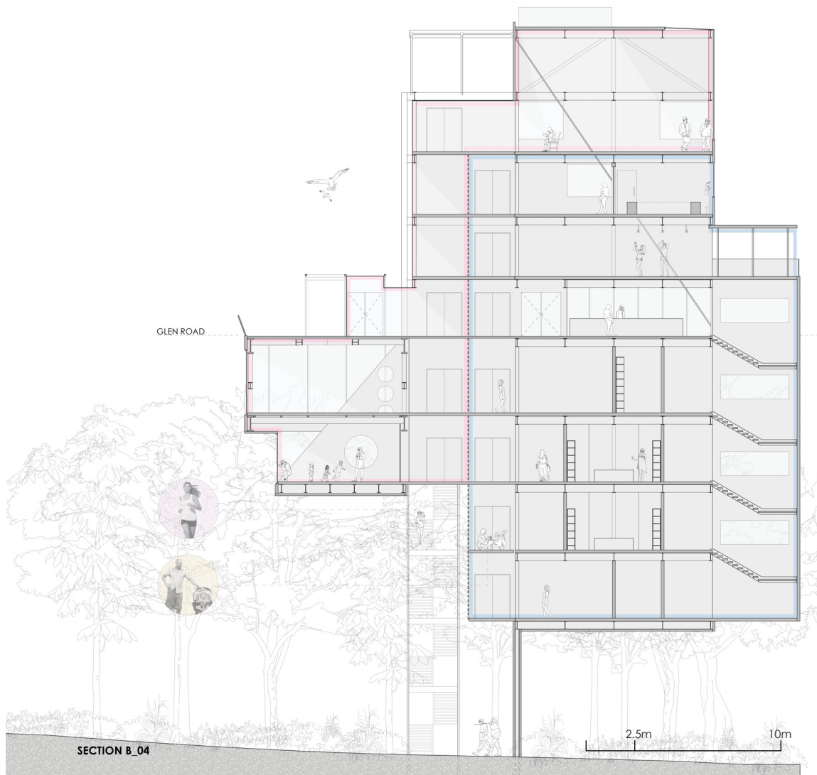
Section facing North: through suspended reading room, shared staircase, and central tower
