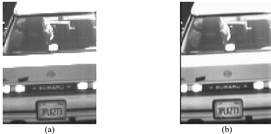
Figure 5.3 Low resolution frame of moving car sequence (1/10). Only 10 frames out of 64 were processed in the region of license plate to reconstruct super resolved image. Improvement of resolution is visible where an unreadable license plate reads “ 3PLK273 ”, as well as the car model reads “ SUBARU ” proving improvement of resolution. This is one of the powerful applications of super resolution shown by our fast working algorithm where it is useful. This image was computed in 0.51 seconds. The LR images are of size 72 \times 121 pixels and reconstructed image is of size 216 \times 363 .
