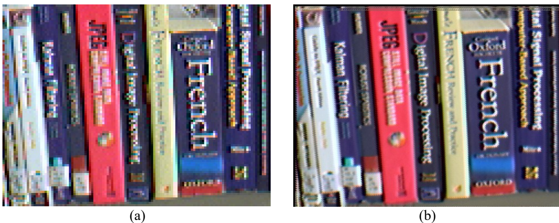
Figure 5.7 Low resolution colour frame of books (1/30) shown in (a) and reconstruction result shown in (b). The gain in resolution is visible through readable titles of the textbook. Some of unreadable texts such as Kalman Filtering, Robust Statistics and the book on the right “Digital Signal Processing” with subtitle “Computer Based Approach”. This result shows that our algorithm works great with colour images as well. The input image is of size 121 \times 91 pixels and output image is of size 484 \times 364 pixels with resolution improvement of factor of 4.
