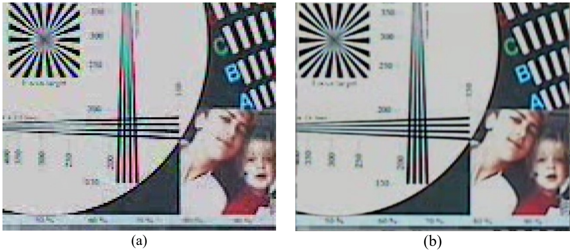
Figure 5.8 Low resolution Adyaron image (1/40) shown in (a) of size 138 \times 115 pixels and super resolved image obtained by our method shown in (b). The resultant image is of size 414 \times 345 pixels.
