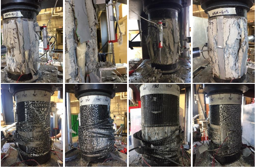
Figure 4. Failure modes - Courtesy of Pedram Sadeghian
