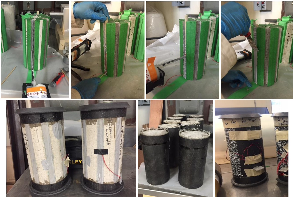
Figure 2. Hybrid strengthening procedure - Courtesy of Pedram Sadeghian
