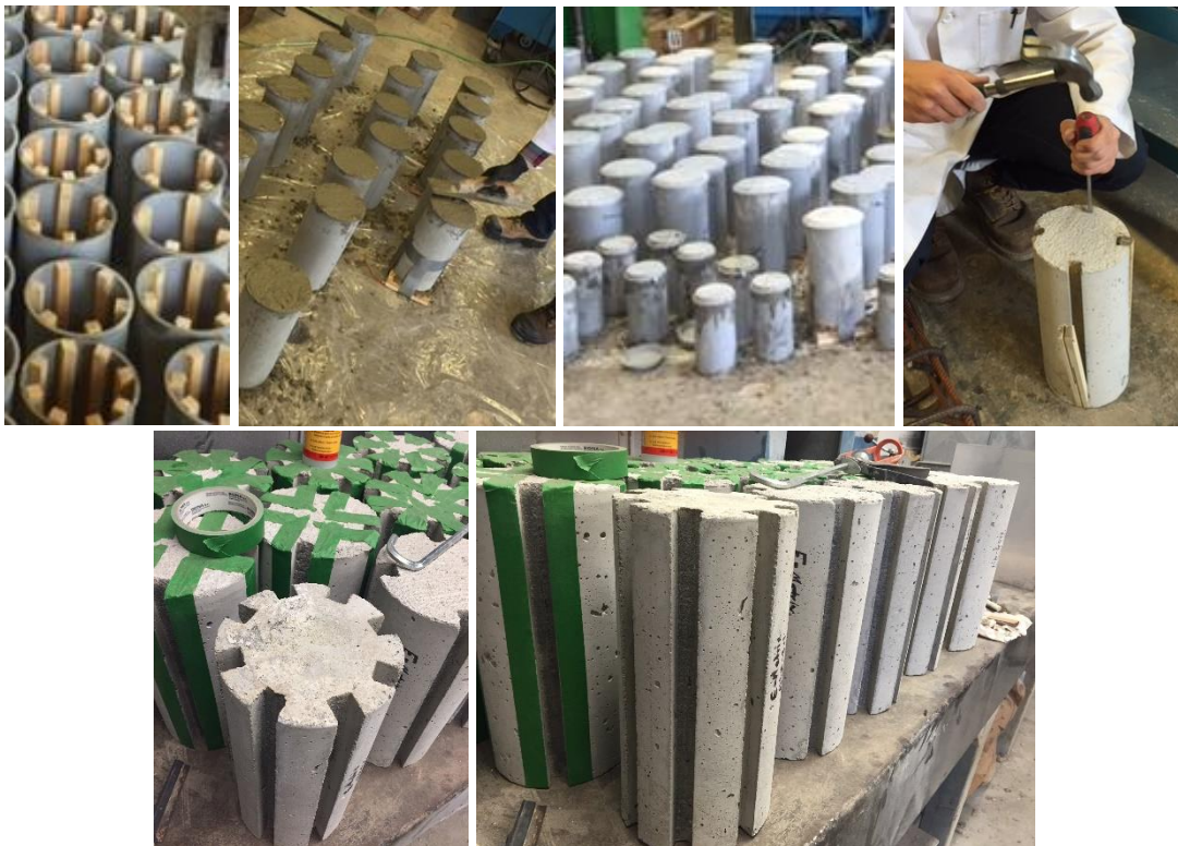
Figure 1. Specimen fabrication - Courtesy of Pedram Sadeghian
