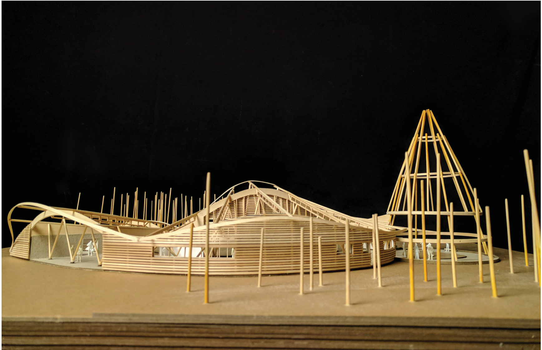
Structure and skin model; view from the north showing the tamarack board rainscreen facade, which can be repaired and replaced as needed.
