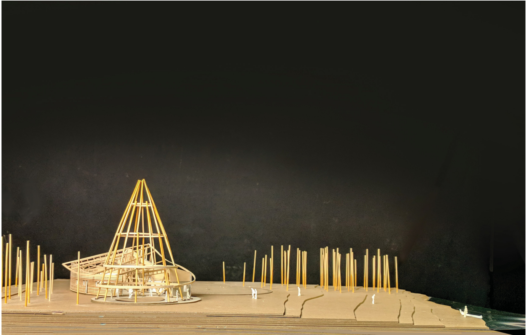
Structure and skin model; view from the west showing how the cone structure shelters the rest of the building from strong winter winds.
