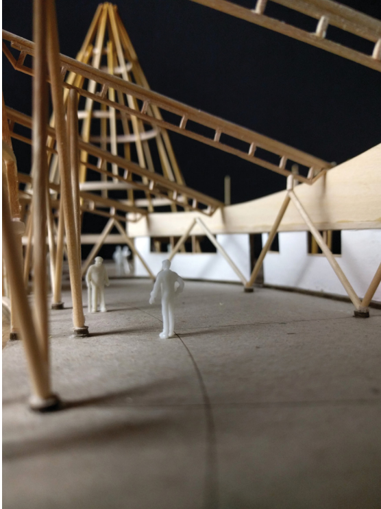
Structure and skin model; view inside the market space and main circulation path.
