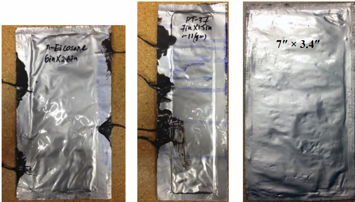
Fig. 4.5 Photographs of three LHTES modules (Ahmed, 2016)
