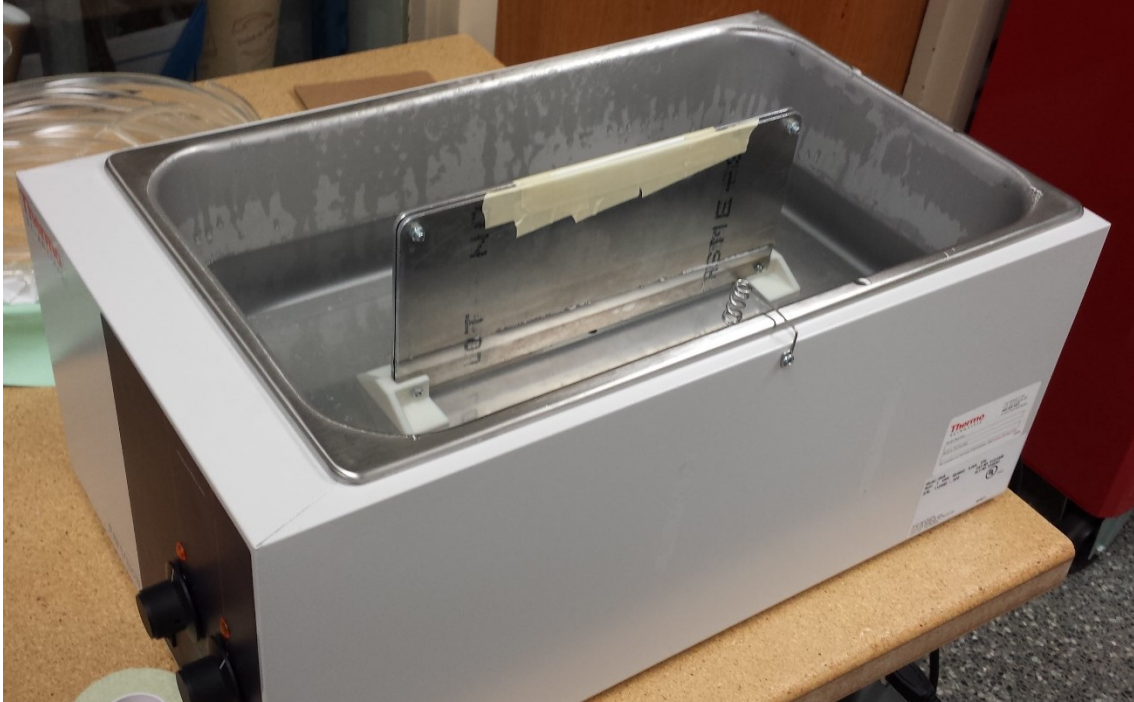
Fig. 5.7 Photograph of the jig with a LHTES package placed in the hot water bath
