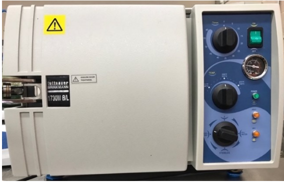
Figure 3.2. Manual Autoclave Dental Steam Sterilizer (Brinkmann Tuttnauer 1730M-B/L) used in the study.
