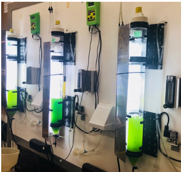
Figure 3.1. 2.25L Tubular PBR culturing system of Haematococcus pluvialis .
