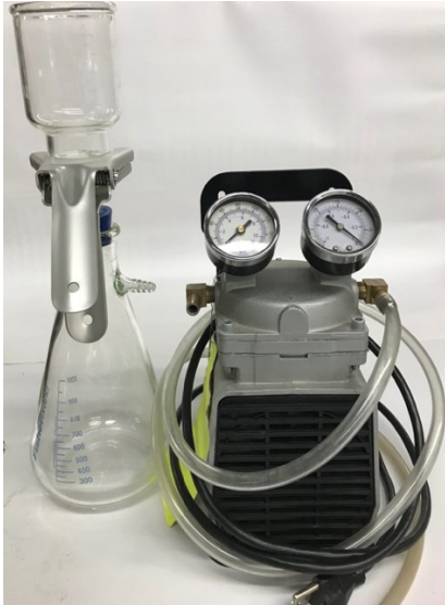
Figure 3.9 Millipore filter assembly and the vacuum pump used in the study.
