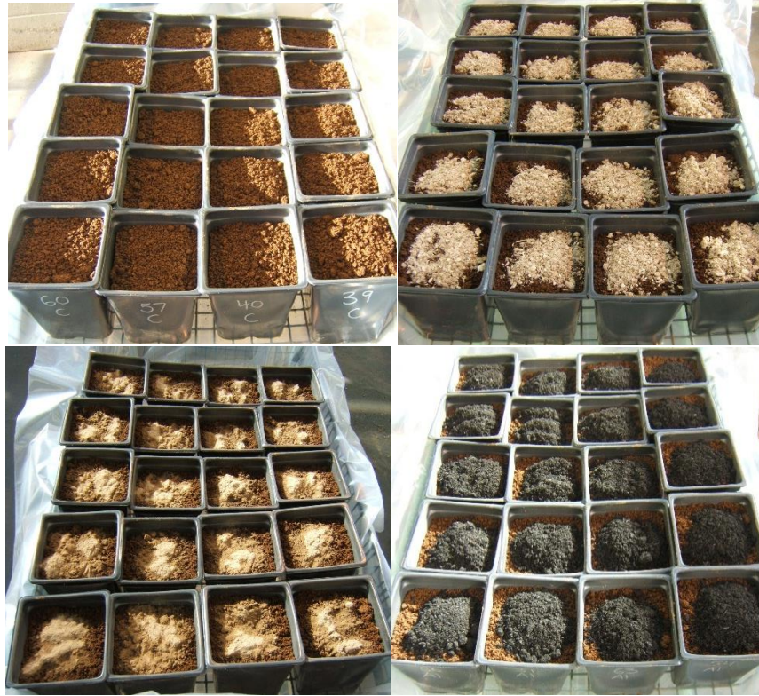
Figure 6.1. Sample soil pots before incorporation of amendments. Clockwise from top left: control, alkaline-treated biosolids (ATB), fly ash, and powdered lime.
