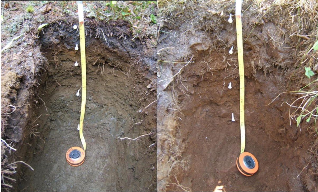
Figure 4.1. Sample profiles for a shaly loam soil derived from slate till (Site 1 - left) and a gravelly/cobbly sandy loam soil derived from granitic till (Site 2 – right). Both soils are classed as Orthic Humo-Ferric Podzols (SCWG 1998) or Typic Haplorthods (USDA 1999).
