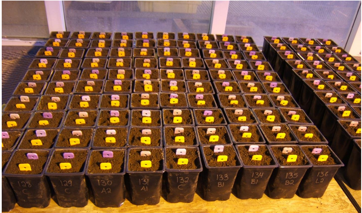
Figure 6.3. Soil 2 treated pots with PRS TM -probes. Each pot was numbered and labelled by treatment as shown in Figure 6.2.
