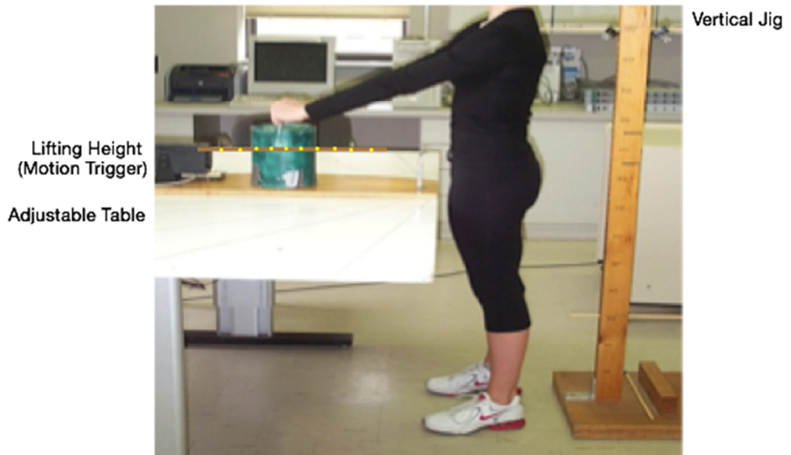
Figure 3. The experimental set-up and lifting height required for the two lifting conditions. Note that the subject is in the maximum reach position and would have their elbows at 90 degrees during the normal reach condition, even though the lifting height did not change for either condition.
