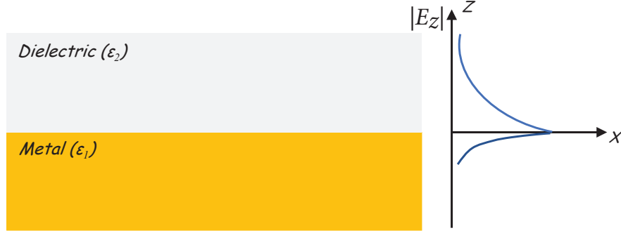
Figure 2.1: Schematic showing interface between two semi-infinite media.
