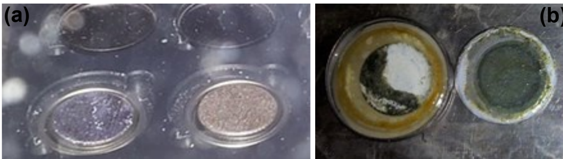
Figure 8.1: (a) Potassium (left) and sodium (right) punched metal foil prior to cell assembly. (b) Potassium graphite half-cell opened after two cycles showing the reactivity of the potassium metal (right).
