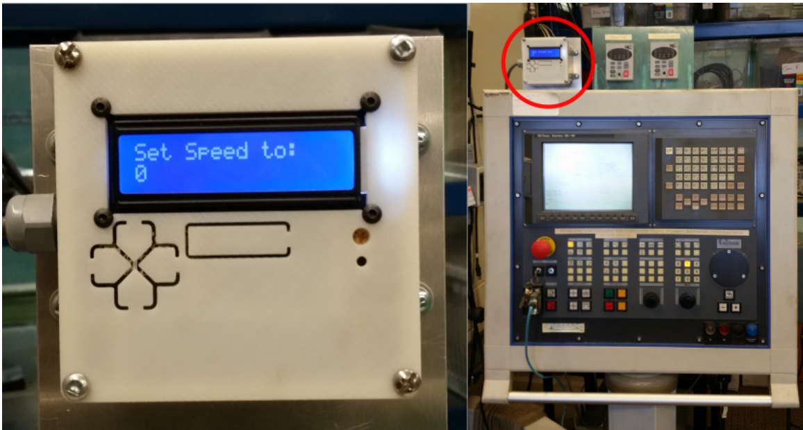
Figure 4.7: The speed controller, left, and its location, right.
