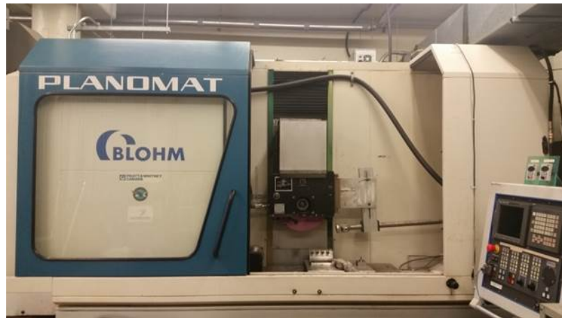
Figure 5.1: Blohm Planomat 408 used for all grinding experiments
