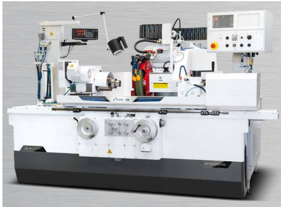
Figure 3.1: A Studer S30 conventional cylindrical grinding machine [23].
