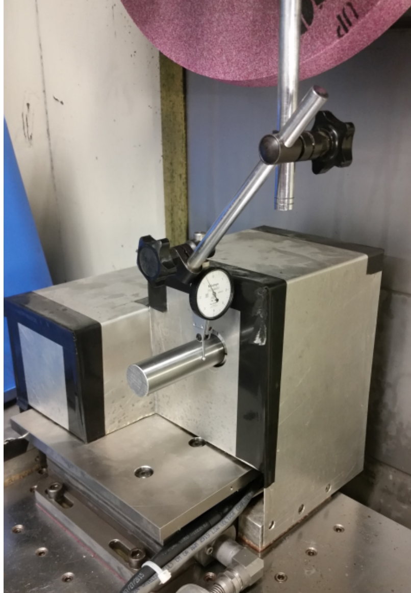
Figure 5.5: The roundness measurement apparatus with Mitutoyo dial indicator
