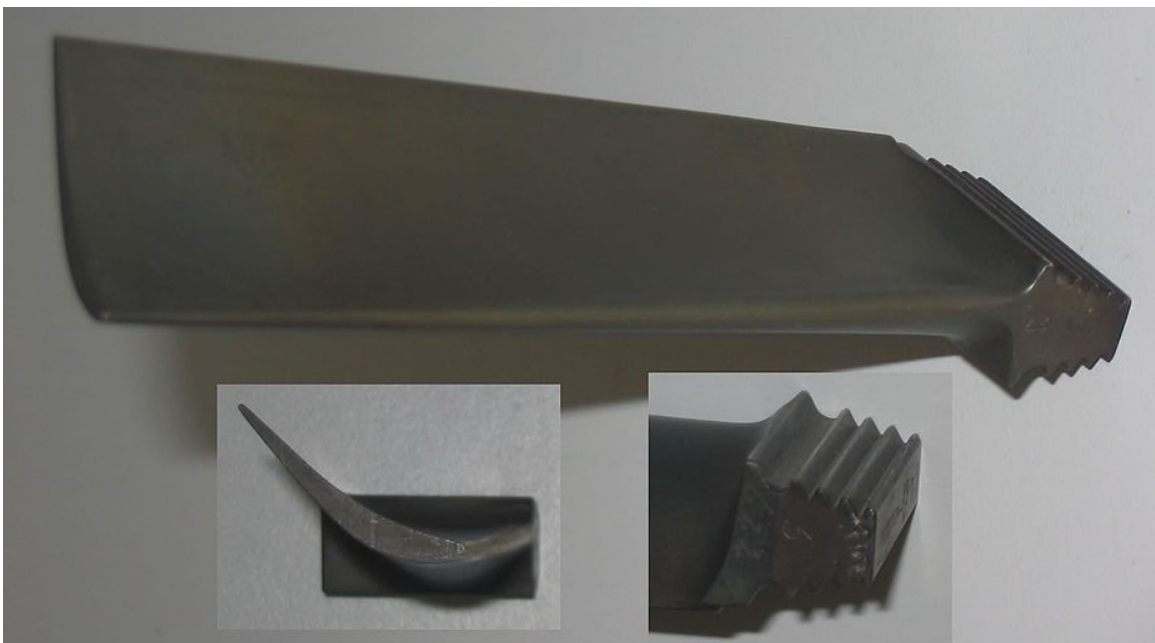
Figure 2.1: An example of a gas turbine compressor blade. The insert on the bottom right shows the turbine root. Image source: Wikimedia Commons [6].
