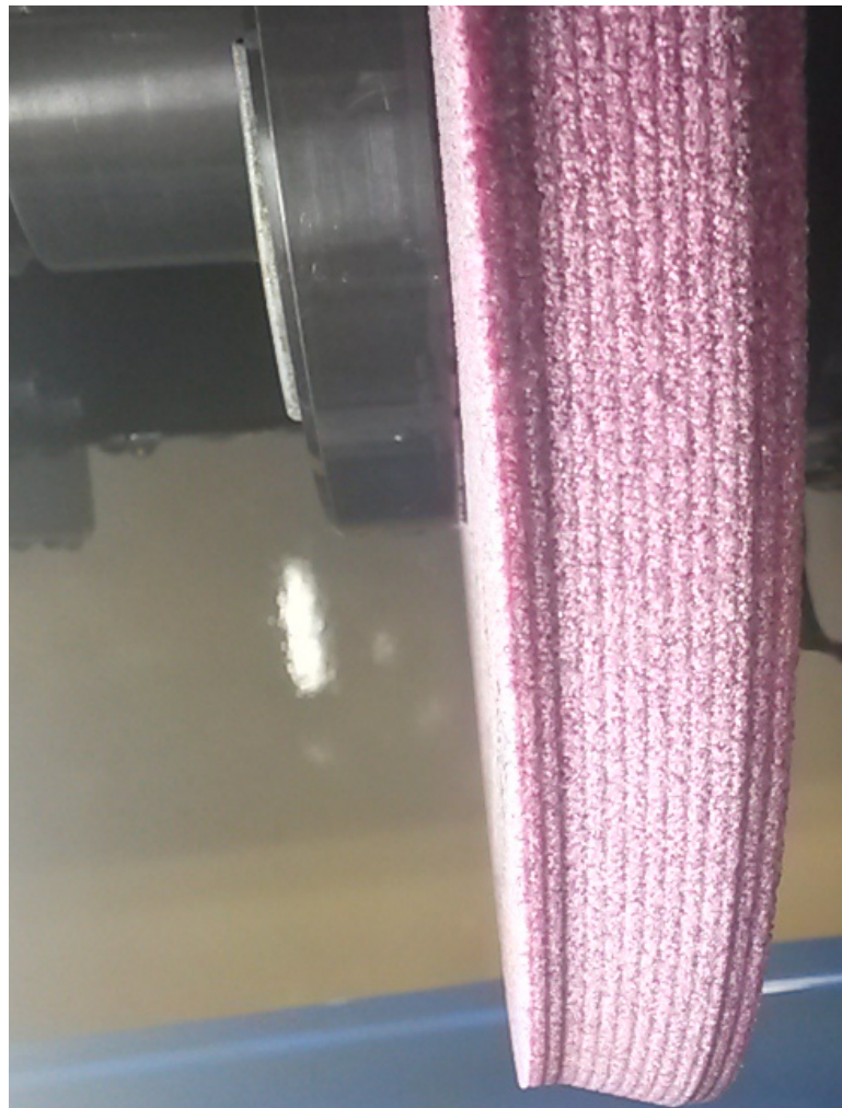
Figure 6.4: Photograph of a grooved profile grinding wheel.
