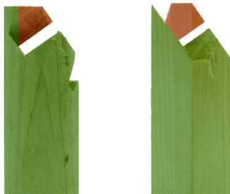
Comparison of the weak point between the original detail on the left to the inverse detail on the right.
