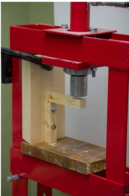
Setup of the acute test showing the jig used to anchor the joint.
