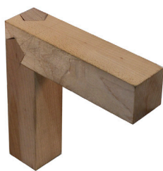
Hand crafted Kawai-tsugite joint shown in its three different positions.
