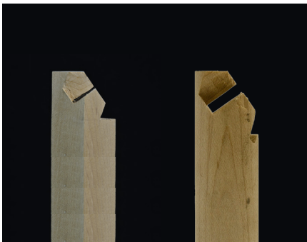
Showing the greater void left by the tooling of the CNC machine (on the right) compared to the little void left by the pull saw blade (on the left).
