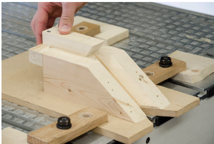
Placing the stock positioner on the jig.
