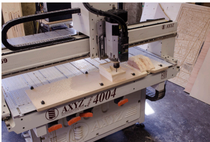
Milling the jig stock material to hold the part stock.
