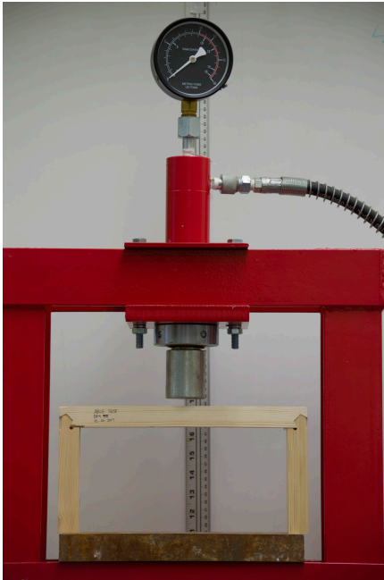
Frame in press, ready for testing.
