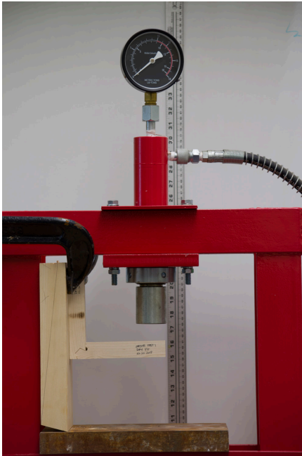
Setup to test the obtuse joint.
