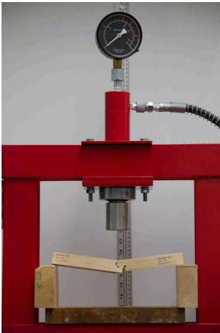
Aftermath of the point load applied to the straight spruce joint.
