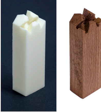
A 3D printed rectangular member on the left and a CNC milled member on the right.
