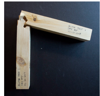
Loaded to failure results.
