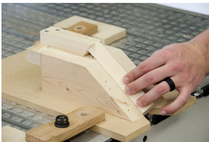
Placing the piece stock against the stock positioner.
