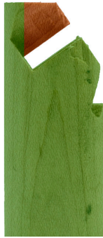
Side elevation representing the strength of the detail: green denotes strength and red denotes weakness.
