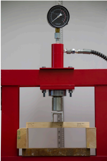
Setup to test the straight joint.
