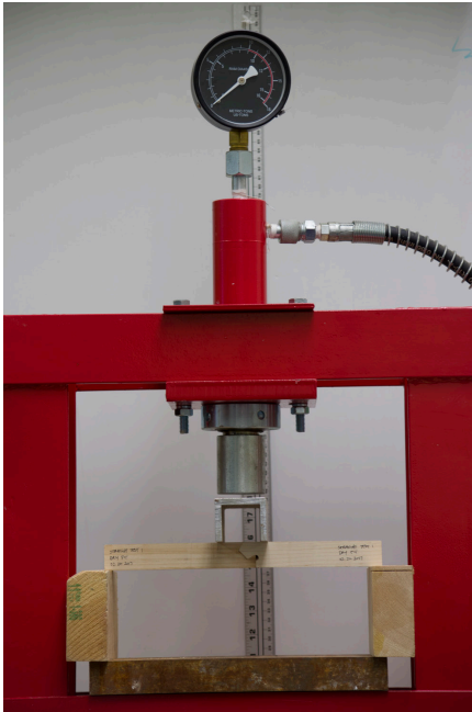
Setup to test the straight joint.
