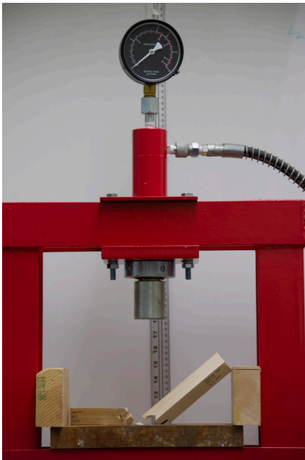
Aftermath of the point load applied to the straight maple joint.
