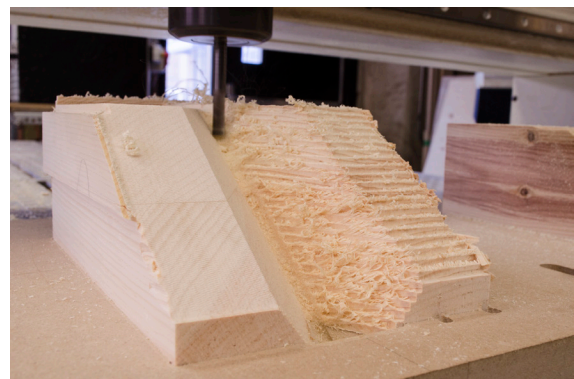
Milling the final surface of the jig.
