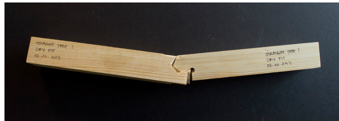
The results of the joint loaded to failure.
