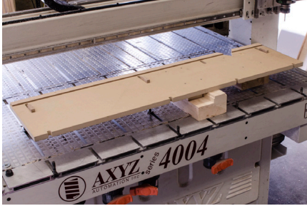
Jig overturned showing aligning pieces and jig stop.
