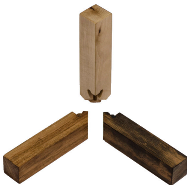
The components of the 3-way joint.
