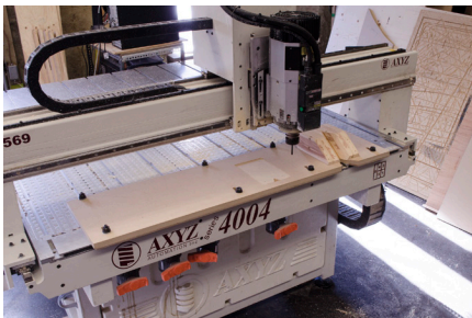
Milling the MDF base for the jig stock material.
