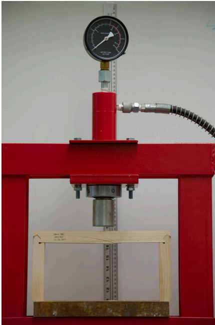
Frame in press, ready for testing.
