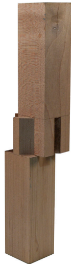
Horizontal movement in the Shihou-hozo-tsugi joint.
