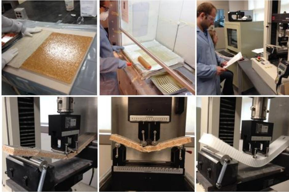
Figure 2: Specimen preparation and test setup
