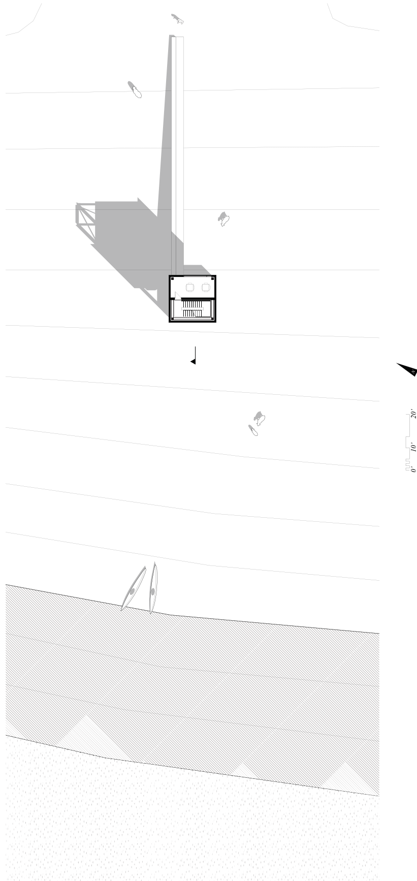
Figure 90 Plan of birding tower illustrating relationship with current and future sea levels
