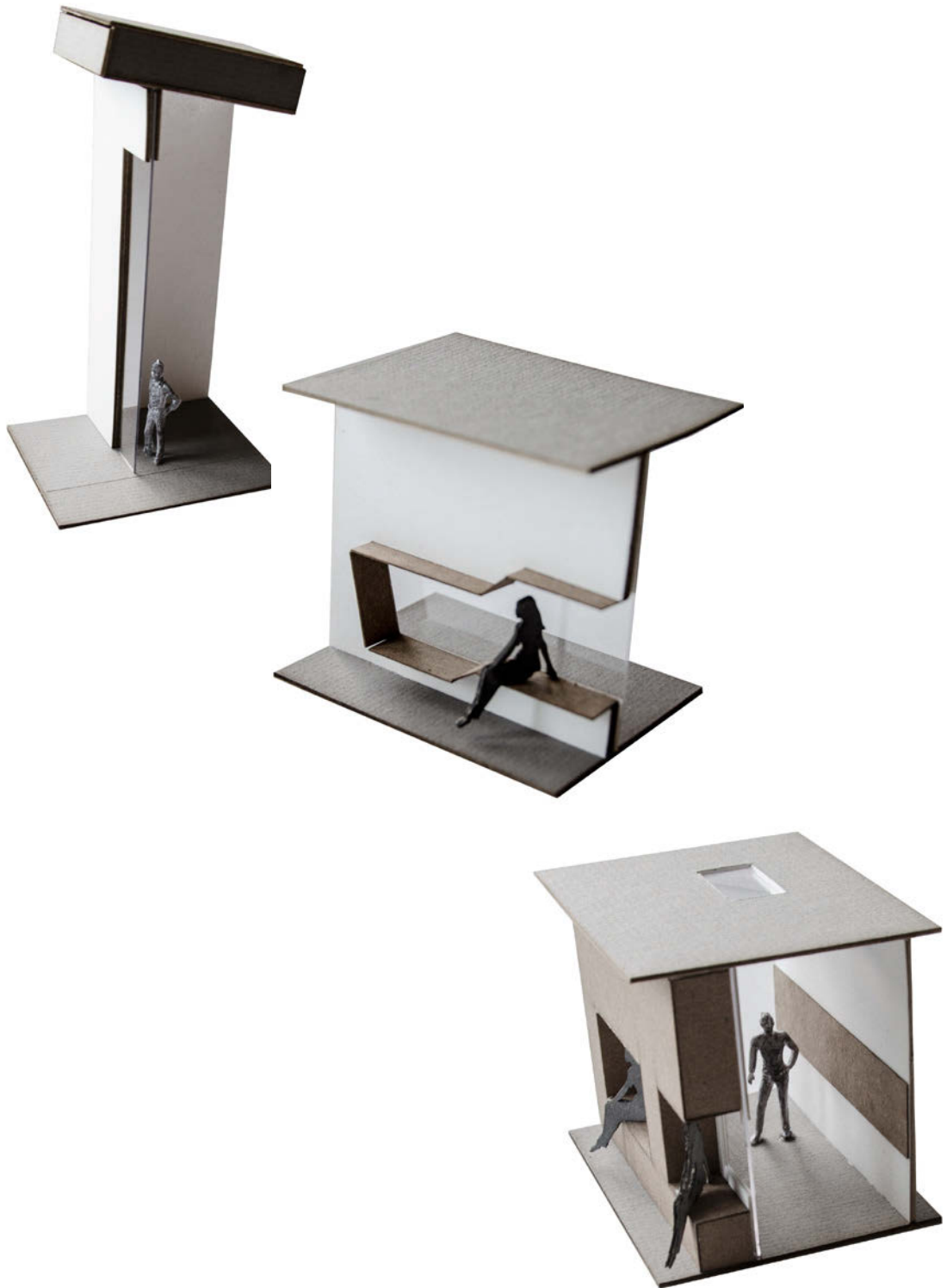
Wall Section models of Recreational Facility building. As you progress deeper into the building, the walls become thicker representing a more refuge-dominant space, whereas the walls closer to the outdoors are more prospect-dominant.
