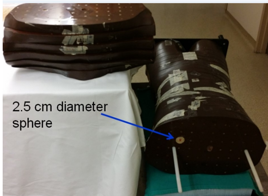
Figure 23 The Rando phantom and the spherical tumor inserted in his lung.
