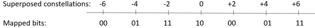
Figure 3.4: The decoding and remapping of 4-PAM symbols corresponding to 1-D in 16-QAM signalling.
