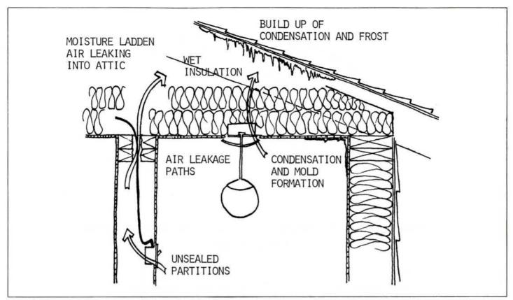
Figure 2. Attic consensation resulting from air leakage through the ceiling.
