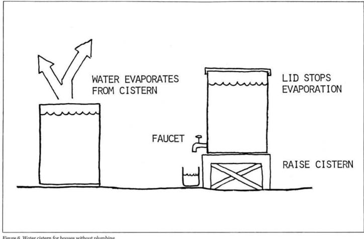
Figure 6. Water cistern for houses without plumbing.
