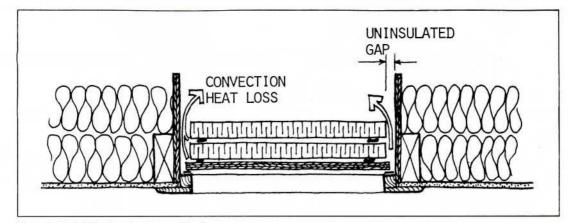
Figure 8. Typical insulated attic access hatch.
