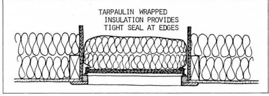
Figure 9. Proposed attic access hatch with good insulation and air seal.
