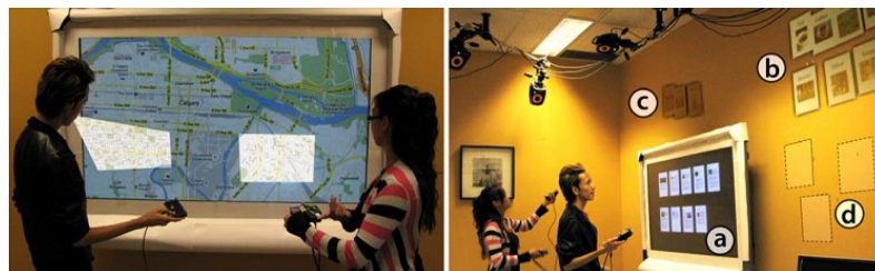
Figure 21 Combining Mobile Projectors and Stationary Display. (Left) Details of map are projected on a large display. (Right) Mobile projectors provided details outside of the screen.
