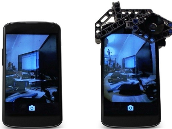
Figure 35 Increasing the FoV by adding a wide lens on the front camera
