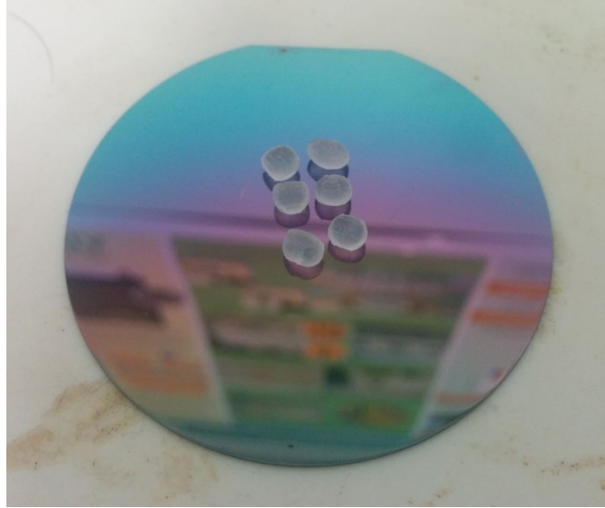
Figure 28: Image of Kraton beads melting on 2" silicon wafer
