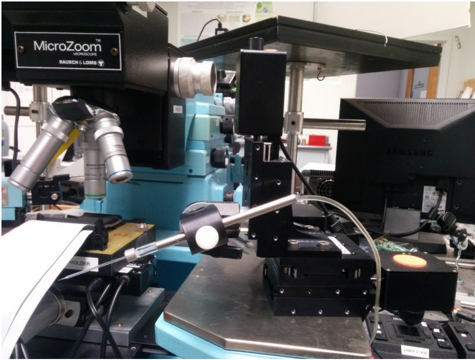
Figure 10: 3DOF system with pipette installed
