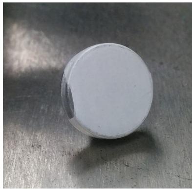
Figure 44: SEM stub covered in Teflon (stub is 13 mm diameter)
