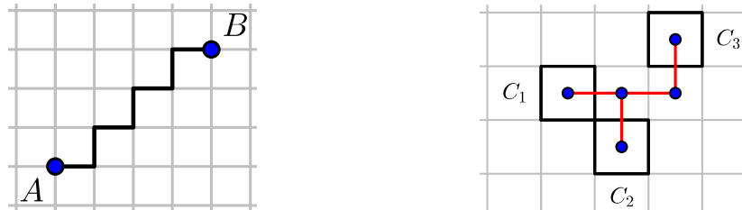
(a) Point A is of 7-cell-distance from point B . (b) C_1 is of 2-cell-distance from C_2 and of 3-cell-distance from C_3 .
